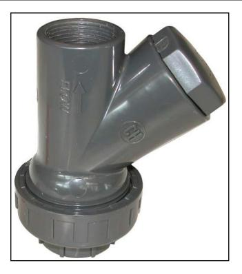
Connection: BSP female threaded version / Solvent socket version Dimensions: threaded ø 3/8" to 3"/ solvent ø 16 to ø 90 mm. Minimal Temp + 0°C Maximal Temp + 60°C Maximal Pressure: 10 Bars Characteristics: Y Check Ball Valve Vertical / Horizontal installation Checking Plug Made of (Material): U-PVC
